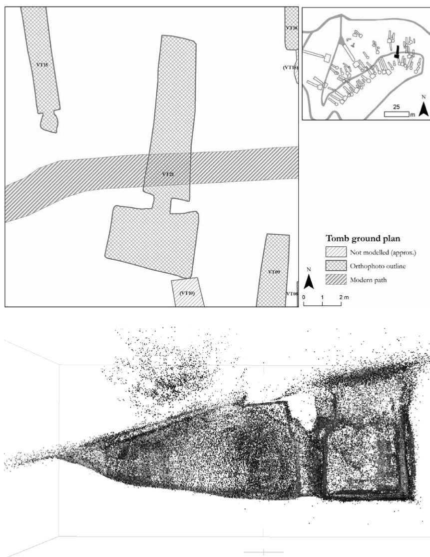
Figure 4.3.12. VT21 ground plan and sparse cloud model (eastern cross-section), showing the extent of its ceiling collapse.
