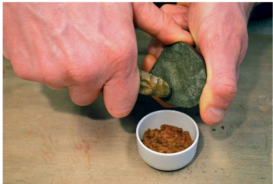
Figure 2: Materials and gesture used for fire-making experiments. The flint crested blade (right hand) was pressed firmly against the flat broken face of the halved pyrite nodule (left hand) and then forcefully pulled upwards to produce showers of sparks that fell into the small ceramic bowl containing the tinder.
