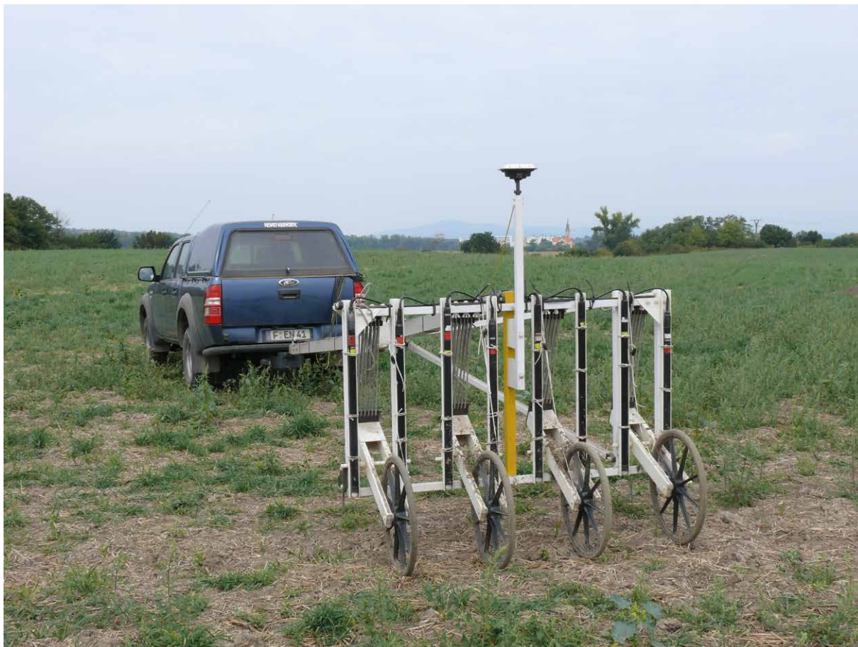
Figure 2.1.3. 8-channel Magnetometer (SENSYS MAGNETO®-MX ARCH) during survey of the 'Fidvár' site in 2008 (photo: K. Rassmann).
