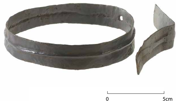
Figure 8.13 Iron bands, probably fittings for wooden water pipes 1:2 (photo Restaura)
