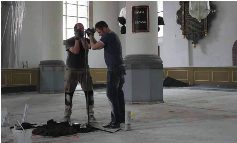
Fig. 28: Core samples being taken inside the Grote Kerk. Photo collection archaeology, Vlaardingen Municipality.
