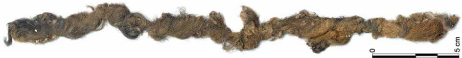
Fig. 13: Oakum consisting of twisted cow hair and sheep's wool. Photo collection archaeology, Vlaardingen Municipality.
