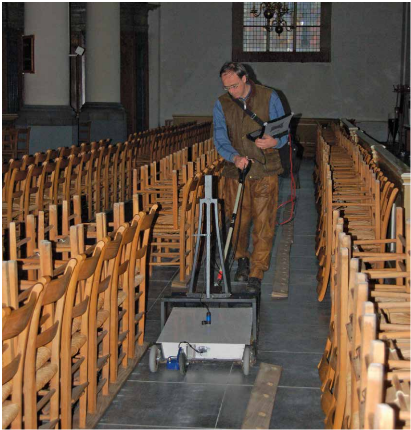
Fig. 27: Using ground-penetrating radar inside the Grote Kerk. Photo collection archaeology, Vlaardingen Municipality.
