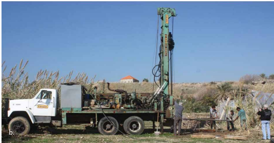
Figure 13. a) Location of auger cores collected in the Armenian Orphanage plot (Nicolas Carayon, 2014); b) auger in action: 291 kg of sediments were cored with 80 kg sampled, processed and analysed in the laboratory. (Photos M. Francis-Allouche & N. Grimal).
