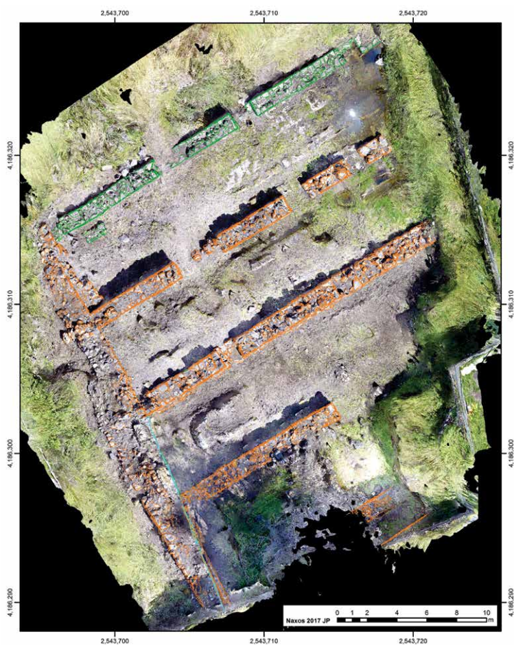
Figure 6.11a (left): Urban Landscape Project of Naxos in Sicily 2016-2017. Shipshed complex. Orthomosaic of the complex with total station data (image by Jari Pakkanen).
