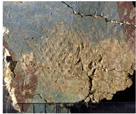
Fig. 18: Floor fragment from room E of the King's Palace. Fine textile impressions visible in the plaster surface and its paint layer indicate the covering of the painted lime plaster floor during the plastering and painting process to ensure proper carbonation.
