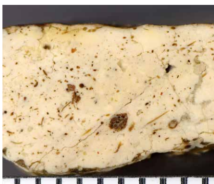
Fig. 15: Cross section of painted dais plaster from palace room F with fine brownish organic plant fibres and shrinking cracks within the mortar matrix. The evenly smoothed plaster surface carries a yellow paint layer with red colour fragments.
