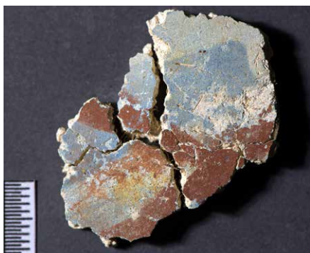
Fig. 13: Painted lime plaster floor fragment from room E. The evenly smoothed upper plaster layer carries polychrome painting and is only 2mm thin.
