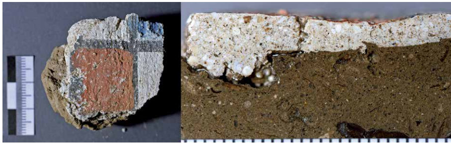
Fig. 10: Fragment of chequerboard frieze with two different plaster types; the cross section shows the first clay plaster layer and a thinner second gypsum-lime plaster that functions as wall painting support carrying the white ground colour with black outlined red and Egyptian blue cubes. Scale 1mm.
