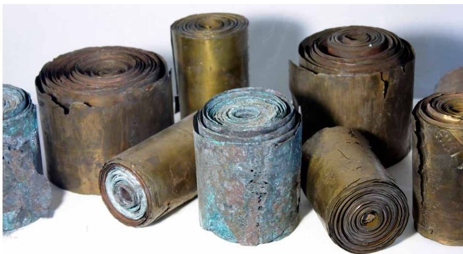
Figure 4: Rolled brass sheet from the Gnalić shipwreck site in the Town Museum of Biograd Na Moru. The diameter of the roll at the center is approx. 7 cm.
