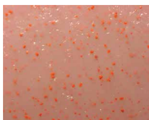
Fig.3 The Raman spectra of vivid red inclusions were found to match with the Raman spectrum of hematite. Clearly, the agate derives its natural pink colour from included hematite.
