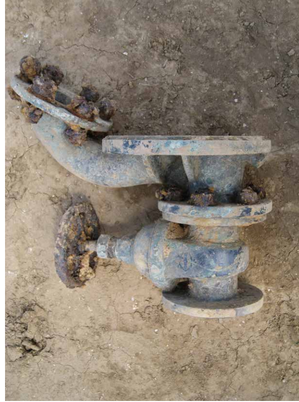
Fig. 4.3. Delivery valve of Livens Large Gallery Flame Projector (© Centre for Battlefield Archaeology, Iain Banks).
