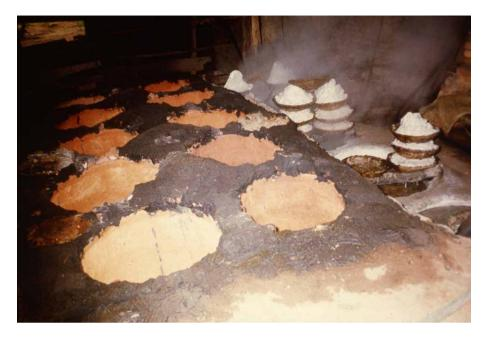
Figure 4. Evaporating brine at the same salt works in the early 1970s. On the left the very large pots known as moyas have been mounted in the furnace and are ready to receive the brine. To the right, granular salt is draining in baskets over metal evaporation pans.
