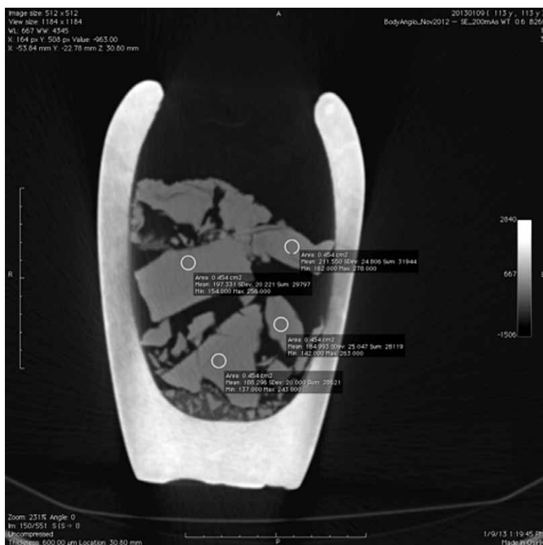
Fig. 1. CT-based cross-section images of a canopic jar (Völkermuseums Burgdorf, Inv. BU_53_07668; Siemens Somatom Definition Flash 512x512 matrix. 0.6mm slice thickness, 120KV, 140mA) (image: IRM, Institute of forensic medicine, University of Zurich).
