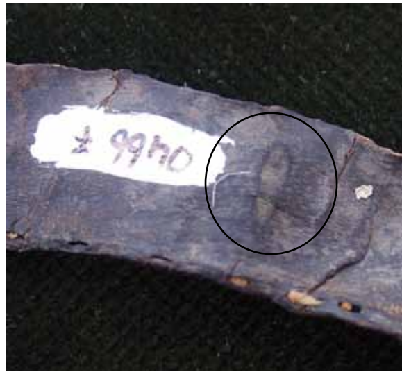
Figure 4. A) A dark spot indicates vegetable tanning (asw-0426i); B) A weak spot is interpreted as ‘unclear’ and vegetable tanning is questionable (asw-0466f).
