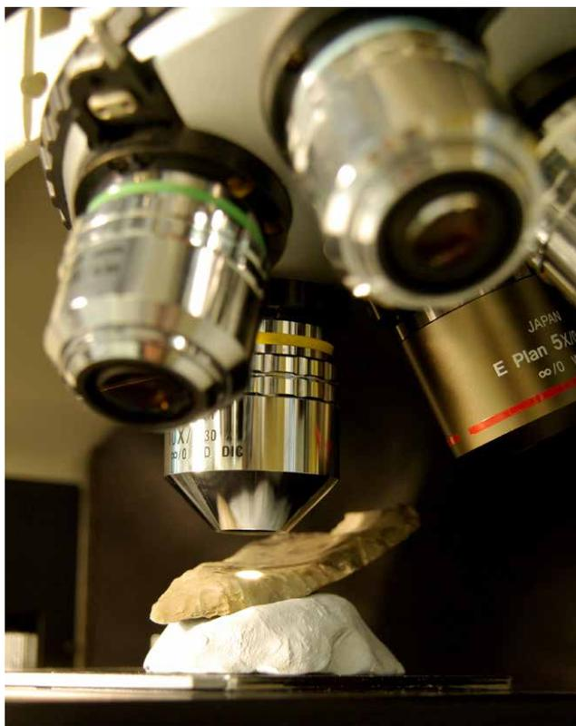
Fig. 1.2 Focus on flint: the use of the metallographic microscope for studying polish and striations under magnifications of up to 560x.
