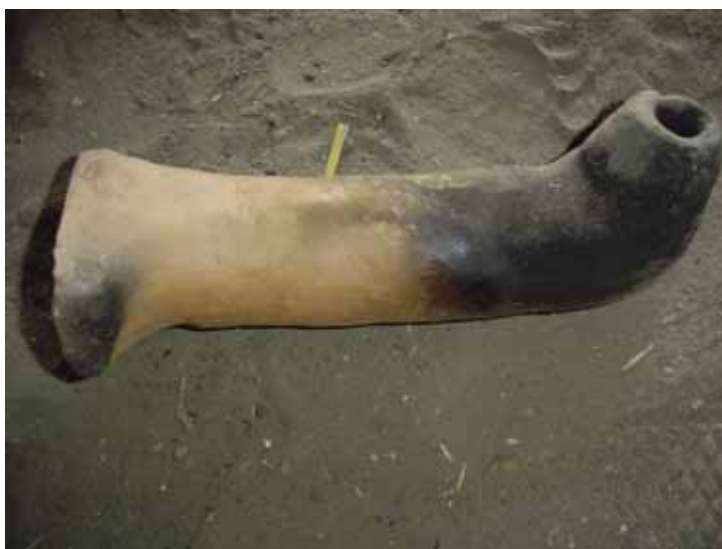
Figure 7.5 The elbow tuyere from experiment 1 (photograph by author).
