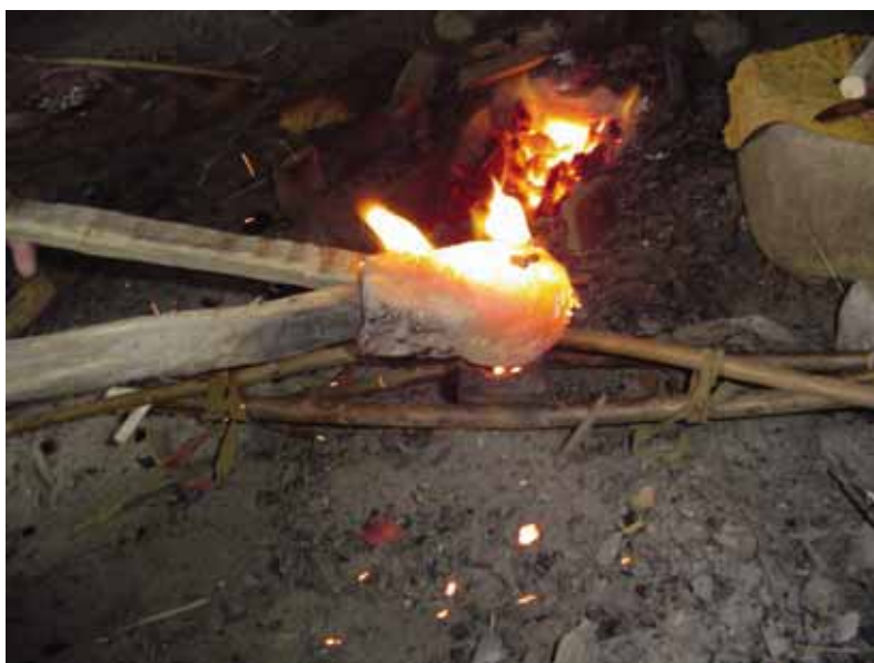
Pouring the liquid bronze in the mould. The stick is used to prevent pieces of charcoal to clog the mould. The mould is held in place with whitties and placed at a slightly sloping angle (photograph by author).
