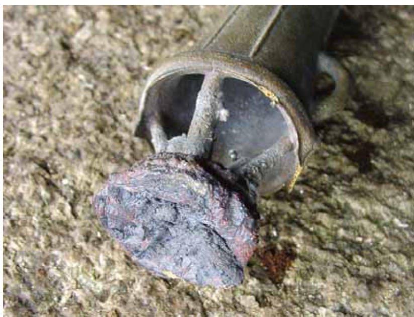
Figure 7.9 A casting jet; still attached to the mouth of an experimentally cast socketed axe (photograph by J. Zuiderwijk).
