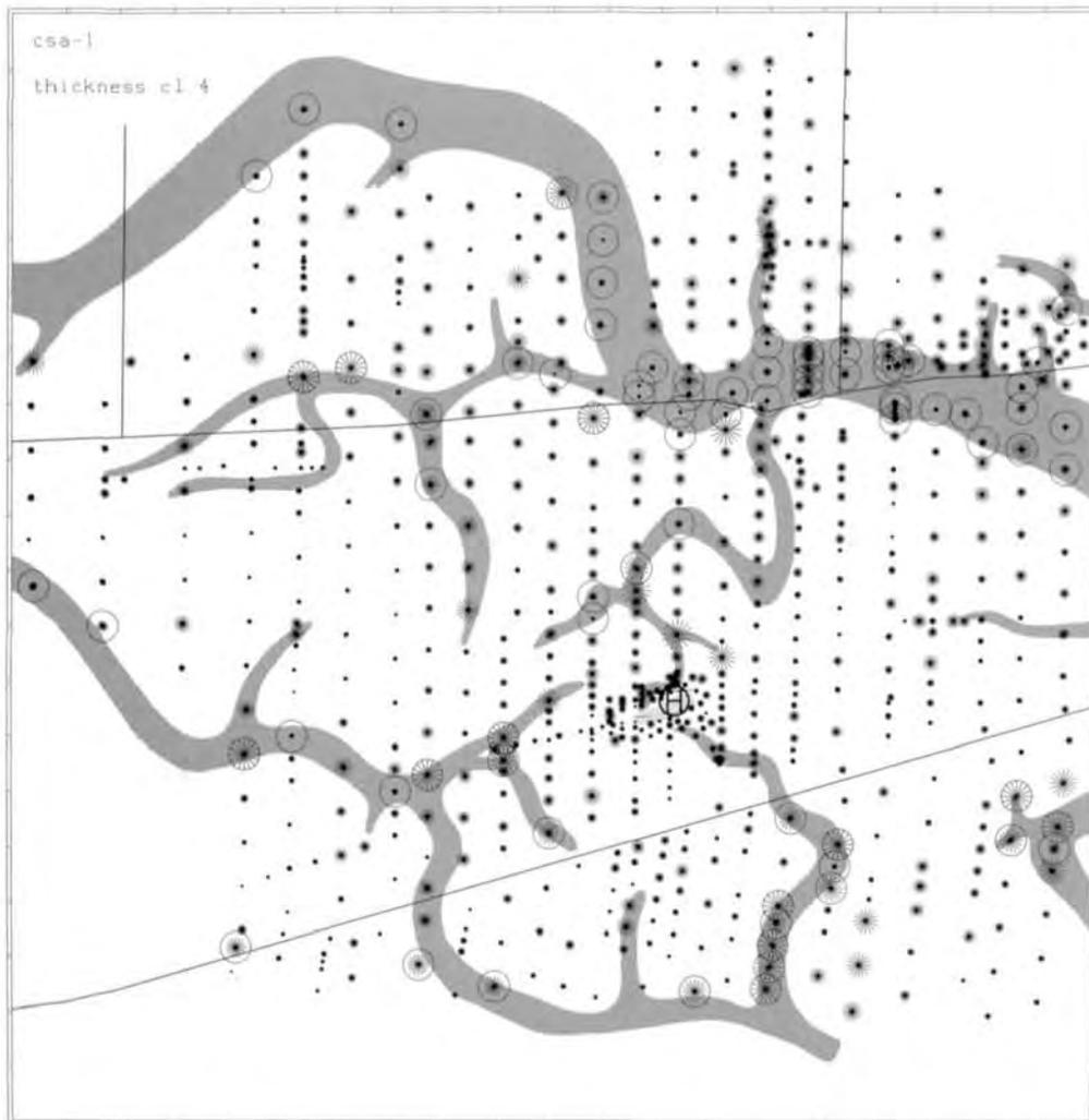
Fig. 51. Thickness of clastic bed cl 4, Molenaarsgraaf. For legend, see Fig. \*35. Dark grey: stream ridges; light grey: river-dune outcrop.
