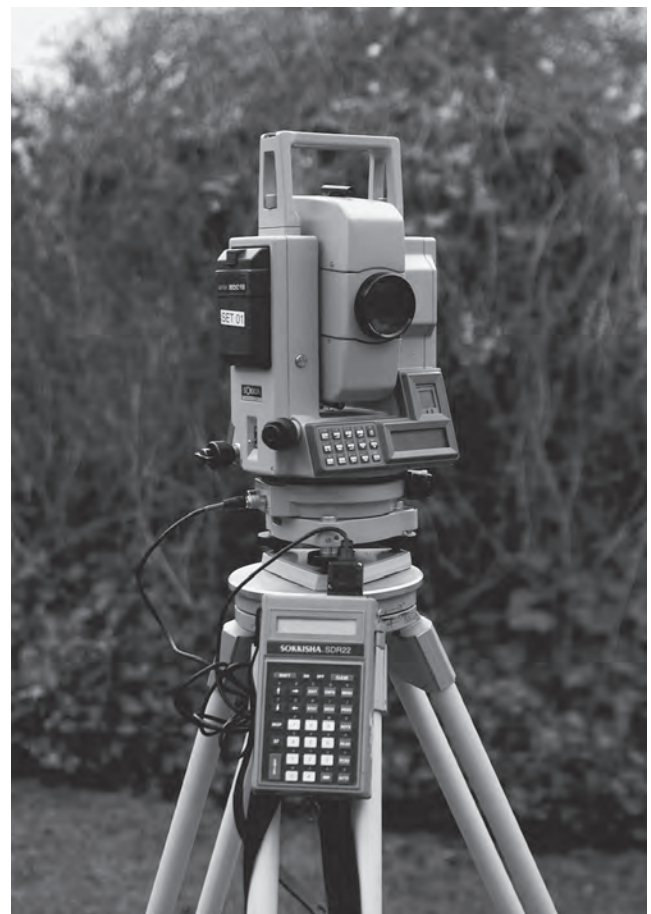
Fig. 2.1 A Sokkia total station set 4B with a survey data recorder (SDR).
