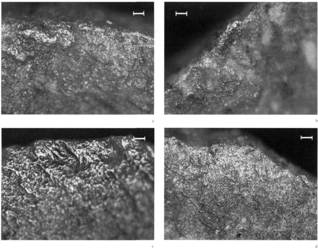
Figure 10. Maastricht-Klinkers: micrographs of traces interpreted as being from contact with wood. All bars equal 50  $\mu$ . a) longitudinal motion artifact nr. 418 (150 $\times$ ), b) longitudinal motion artifact nr. 308 (150 $\times$ ), c) transverse motion artifact nr. 416 (150 $\times$ ), d) wood planing artifact nr. 75 (150 $\times$ ).
