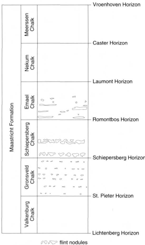
Figure 2. Schematic lithological section of the Maastricht Formation in the Valkenburg region (after Felder et al. 1979).
