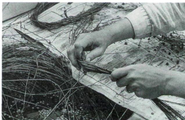
Fig. 19 The loosening of the inner flax fibres from the rotten outer skin; an obtuse-angled tool is used to break and remove the outer layer.
