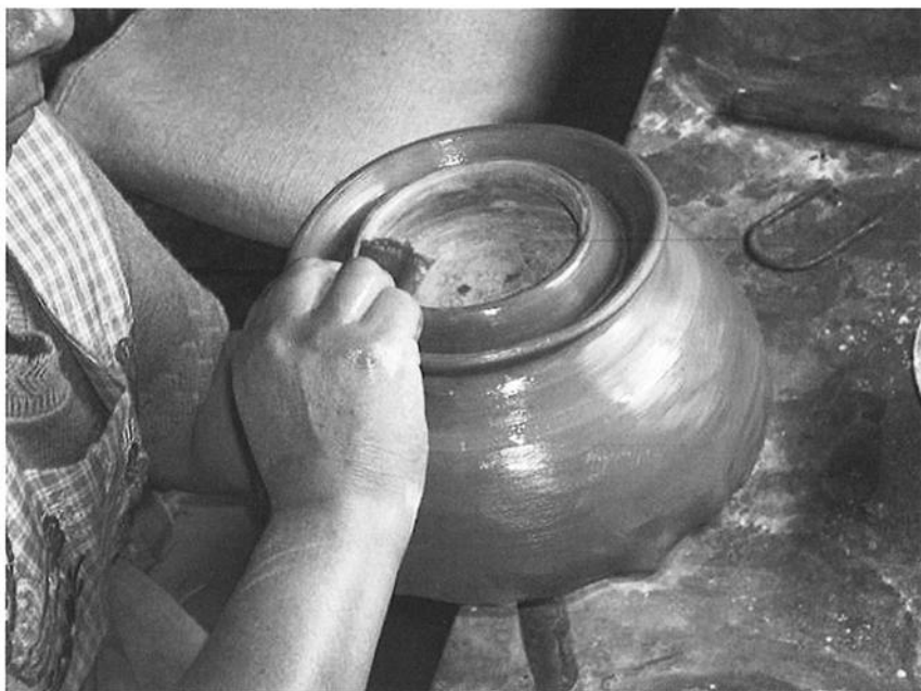
Figure 32. Loosening the clay from the mold to finish and smooth the rim with a wet cloth.
