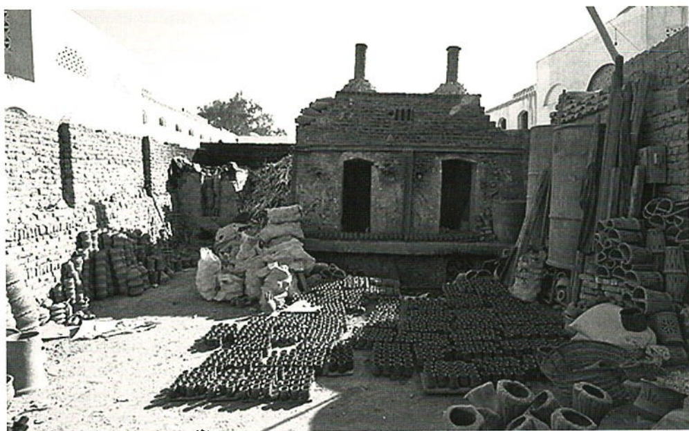
Figure 4. Workshop 1: the courtyard filled with fired and unfired objects. In the background from left to right: a small kiln and two petrol/diesel ovens.
