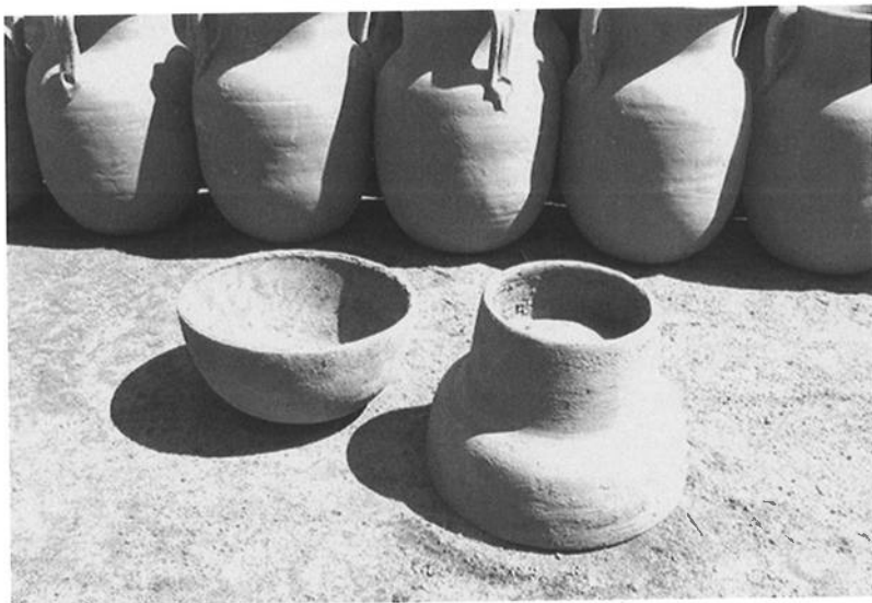
Figure 10. Moulds to make the base and the neck of jars from the workshop of Clemente Sánchez Romero and family in Amozoc. They make the base and the neck of the jar with moulds; then connect both parts, smooth the junctures, make the rim and attach lateral handles.
