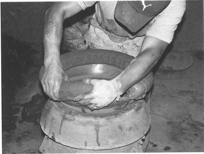
Figure 12. A potter of the family Ramírez Carrillo of Metepec makes the walls of a cazuela by applying a coil on the vessel's base made by moulding.
