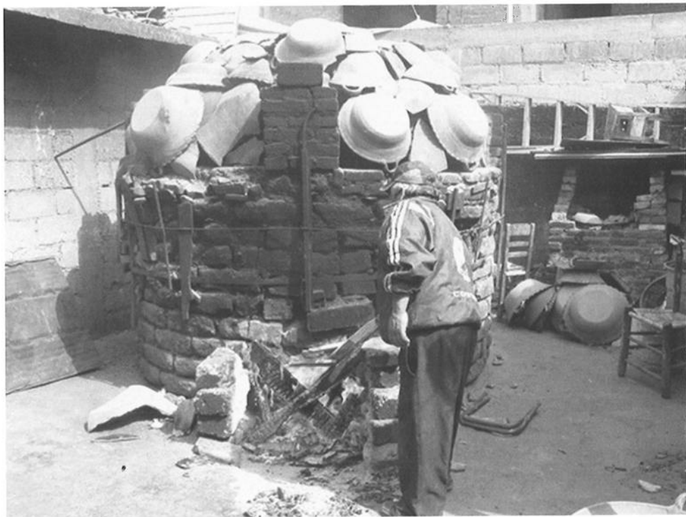
Figure 15. Pots are fired twice in two-chamber kilns, like the one used by the family Torres Carrillo of Metepec. The kiln has an extra chamber for firewood on the bottom.
