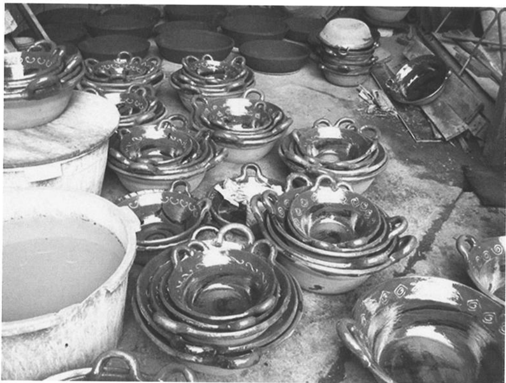
Figure 16. The workshop of Patricio Ramírez Carrillo in Metepec normally produces sets of cazuelas of five different sizes. The vessels are decorated with hasty lines and curves in black glaze, and also with different stamped geometrical motifs in yellow paint. Next their interior is covered with a clear lead oxide glaze and submitted to a second firing.
