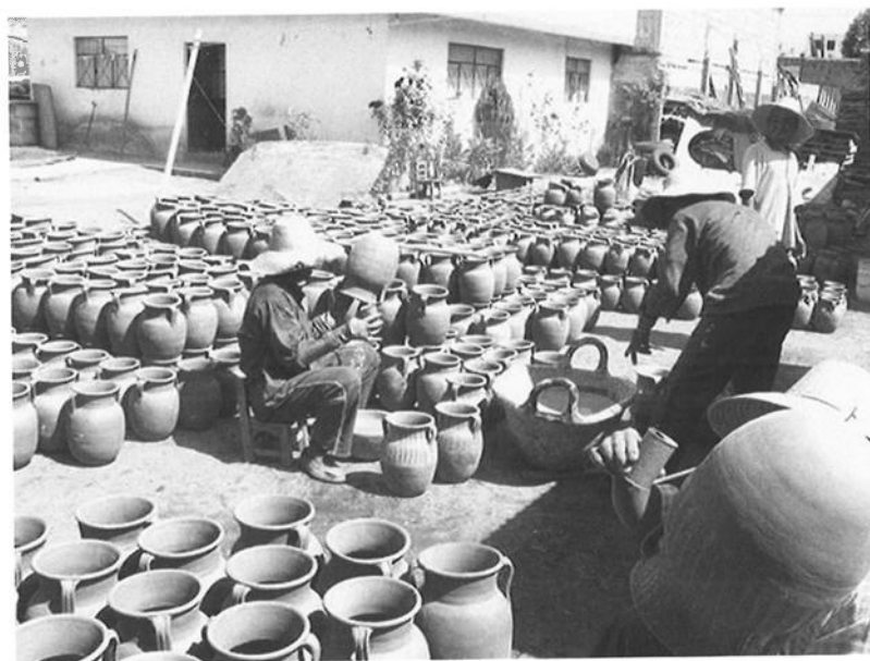
Figure 11. After the first firing, the family Sánchez Romero of Amozoc decorated their jars with hasty lines of black glaze. Then they are covered with a clear lead oxide glaze, and fired for a second time.
