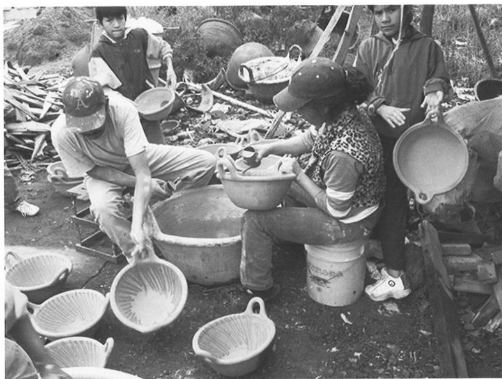
Figure 9. After the first firing, vessels are decorated with hasty lines of black glaze, as is shown in this image of the workshop of Juan Antonio Sánchez in Amozoc. Then they are covered with a clear lead oxide glaze, and fired for a second time.
