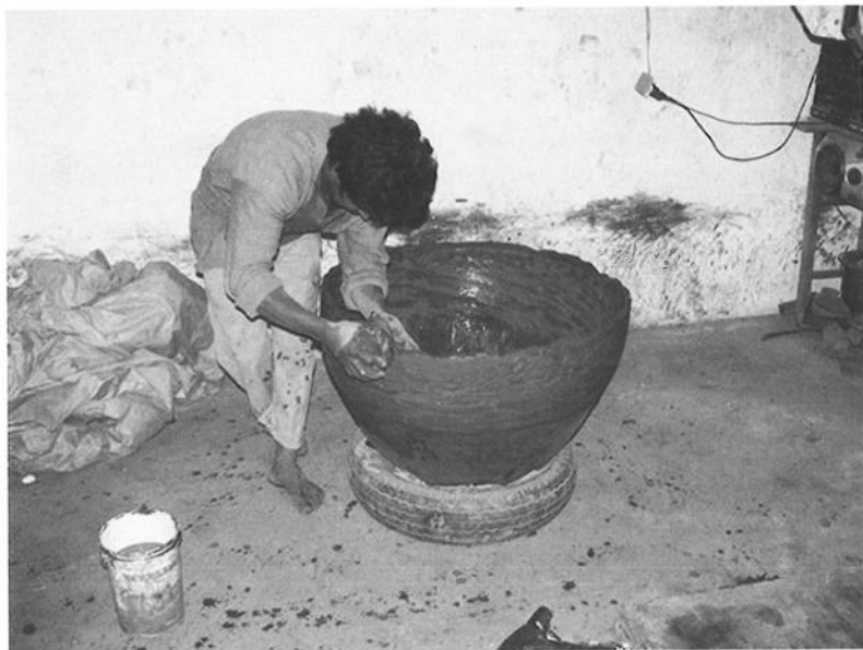
Figure 4. Making the walls of a cazuela in the workshop of Juan Antonio Sánchez and family in Amozoc. Coils are applied on the moulded base of the vessel to build the walls, then they are modeled and polished.
