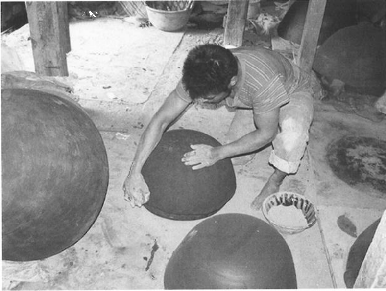
Figure 3. Making the base of a cazuela by moulding in the workshop of Juan Antonio Sánchez and family in Amozoc.
