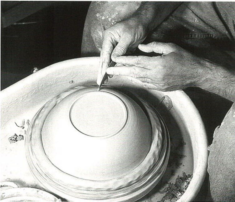
Figure 5. Making a foot stand by scraping while spinning the wheel.
