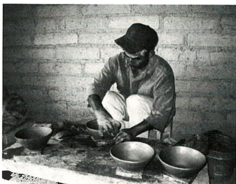
Figure 13d. Making a ko'ò : don Eulogio finishing the brim of the pot with a ñii .
