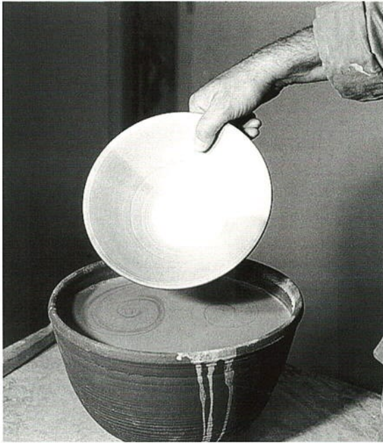
Figure 7. After dipping the other half of the vessel an overlap of the slip coating is visible in the middle.
