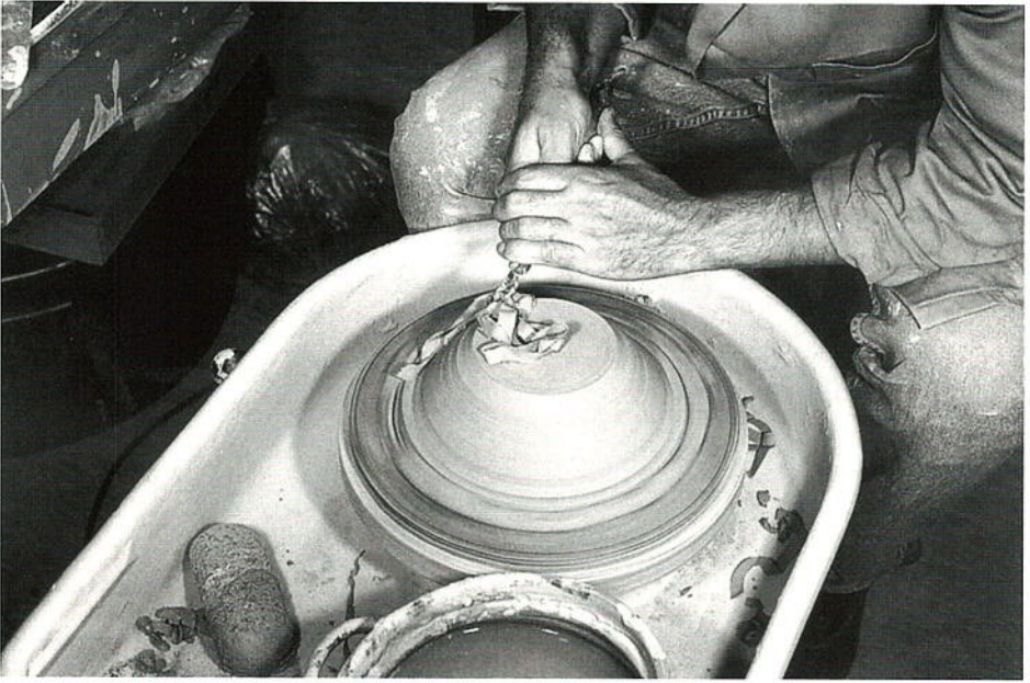
Figure 4. Scraping the outside of the leather-hard vessel while spinning the wheel.
