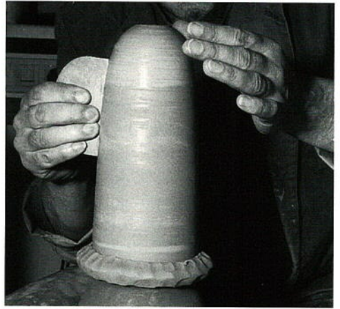
Figure 10. Reducing the wall thickness.
