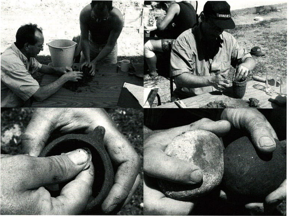
Figure 2. Workability tests on clay samples and the production of test vessels by the Ceramic Laboratory of the Leiden Faculty of Archaeology.
