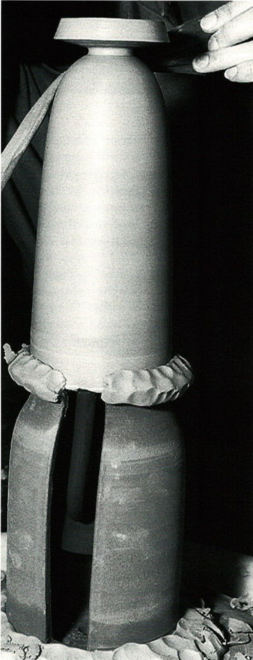
Figure 12. A supporting ring without room for the handle.
