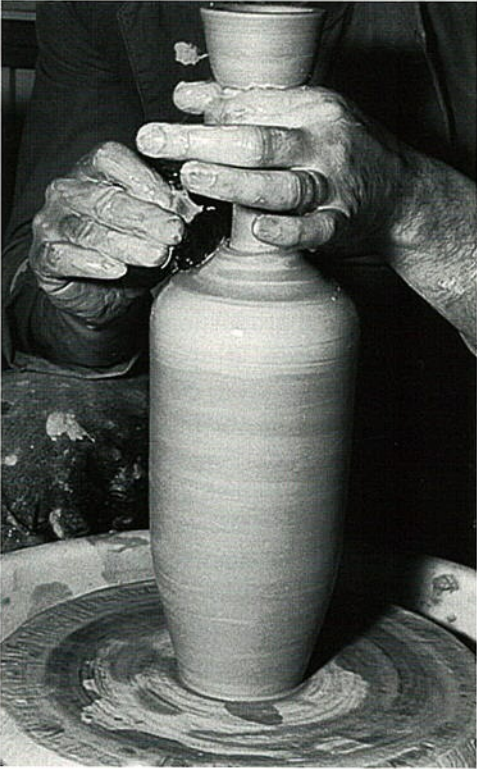
Figure 7. Connecting the neck to the body.
