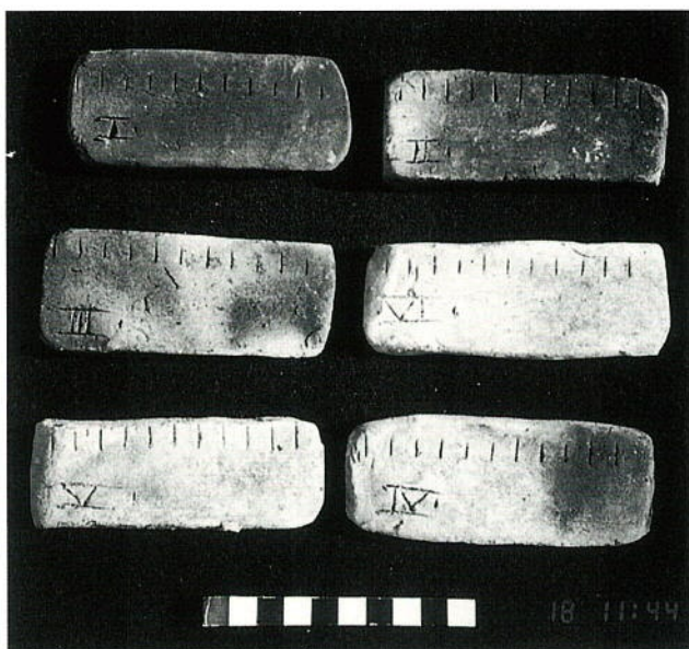
Figure 13. Fired experimental briquettes.
