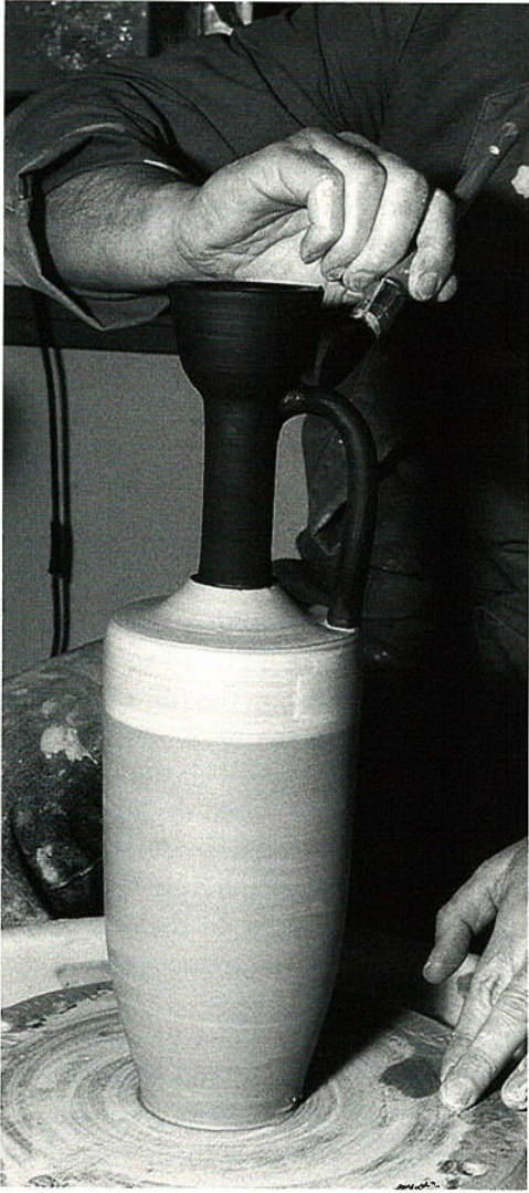
Figure 9. The application of a slip layer
