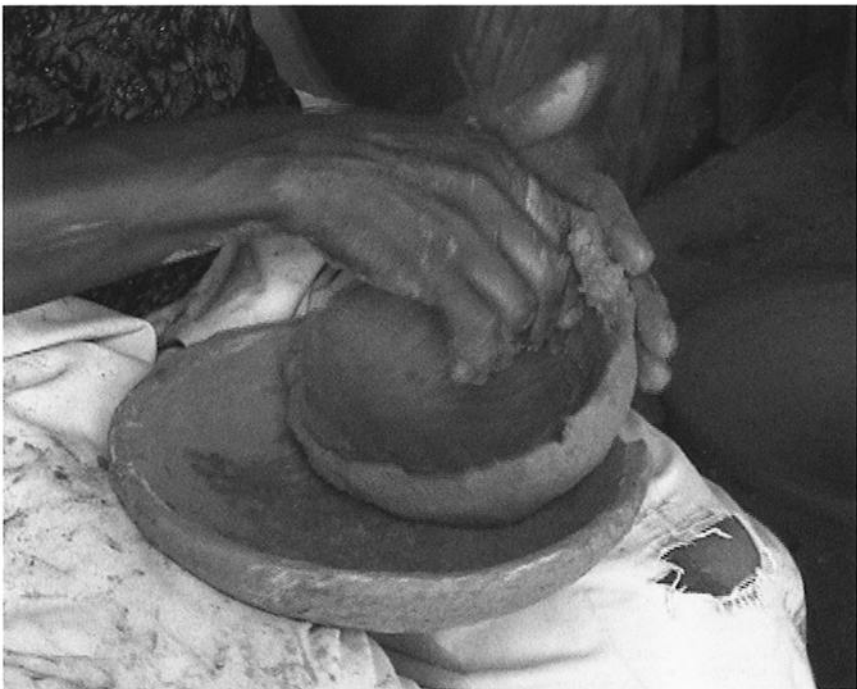
Figure 16. Smoothing out a coil to form the base part.
