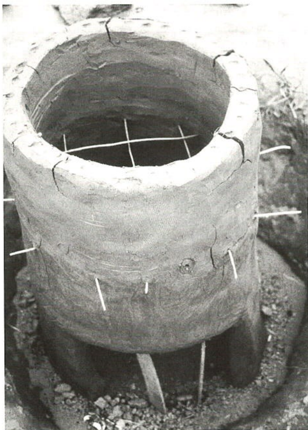
Fig. 4. Experimental updraft kiln. This picture was taken before the firebox was buried leaving an opening to stoke the lower chamber. The stiles in the opening support a thin board that in turn supports the last horizontal coil spanning the width of the opening. The stiles were removed after the coil dried. In order to give the lower section time to become rigid enough to support the next section. The construction took place over three days. The top section, with no salt, has cracked, while lower sections have undergone little distortion with drying. The lower section with salt temper fared much better at this stage, but when fired the section with a larger amount of salt effloresced.
