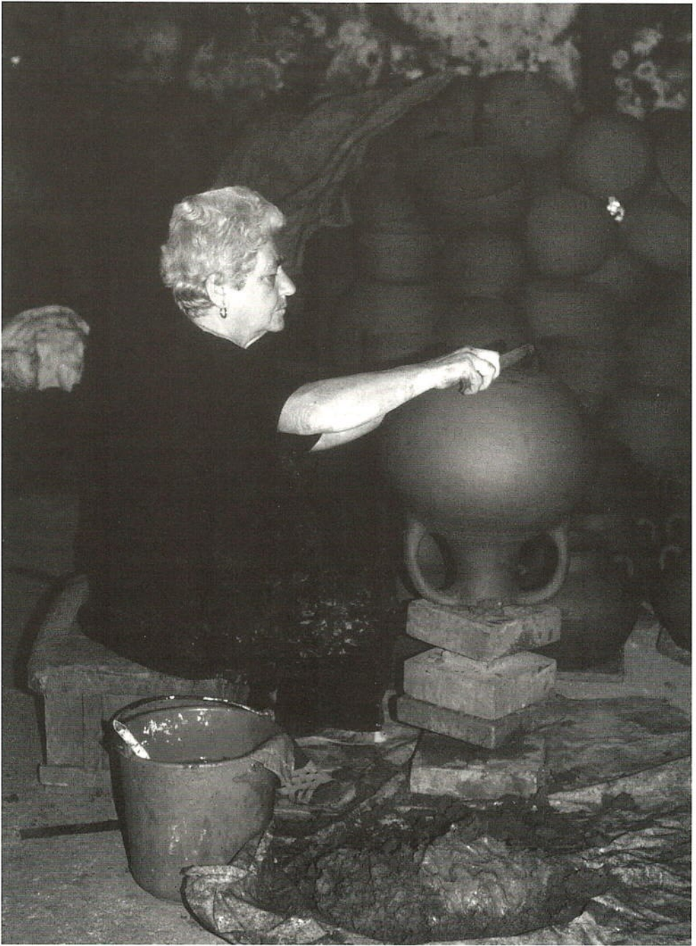
Fig. 3. A Kornos potter in 1999 scrapes the base of a coil built pot that is held upside-down on two wooden turntables. Excess clay removed from the base will be saved for future pots.
