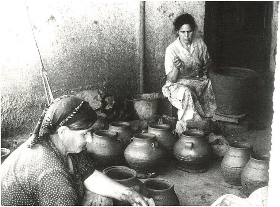
Fig. 2. Two Kornos Pottery Cooperative members making cooking pots in 1986. Only the potter on the right, who is working on the lower part of an oven, was still making pottery in 1988 and continues to do so in 1999. The cooking pots are coil built on a slow moving turntable. Initially the flat bases are left thick and the lower bodies have string wrapped around them to prevent their collapse. Once the upper bodies dry slightly, the string is removed and the bases are scraped and rounded, as seen for a two-handled stamni in Fig. 3.
