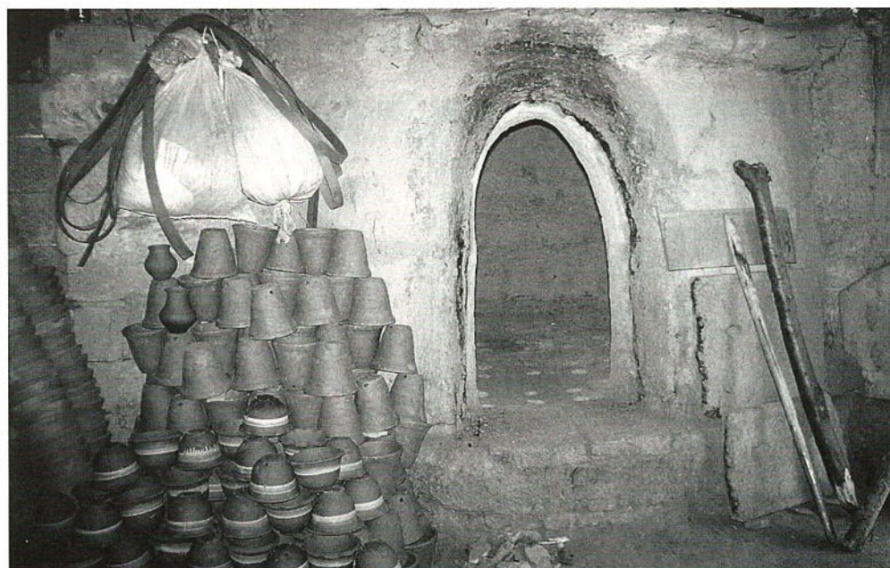
Fig. 6. The entrance of the pottery chamber of the updraft kiln, Örnekköy (Turkey).
