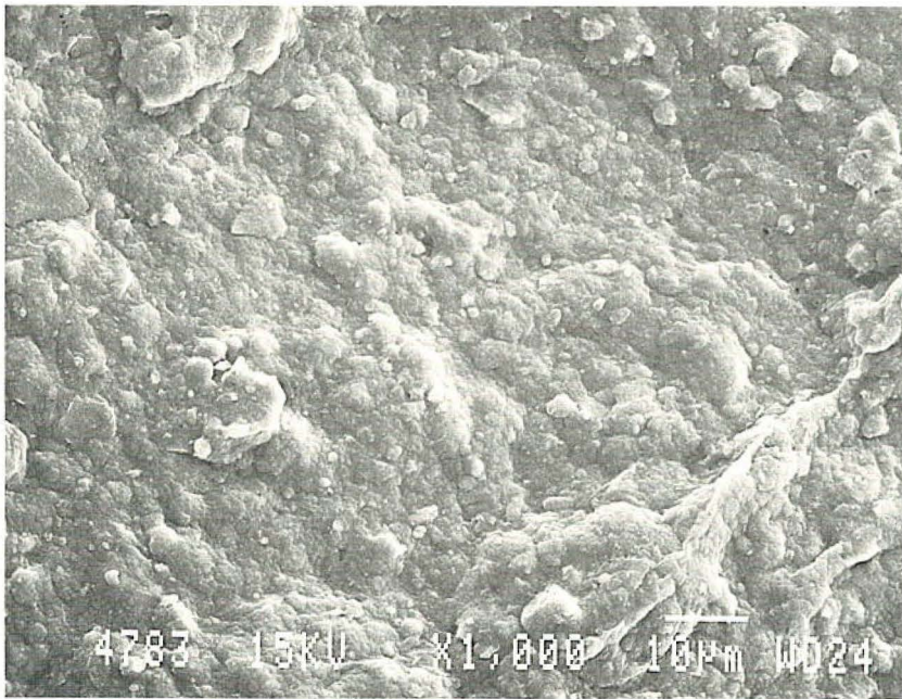
Fig. 5. Electrical scan of the natural clay. Enlarged 1.000x at 15 Kv; scale 10.
