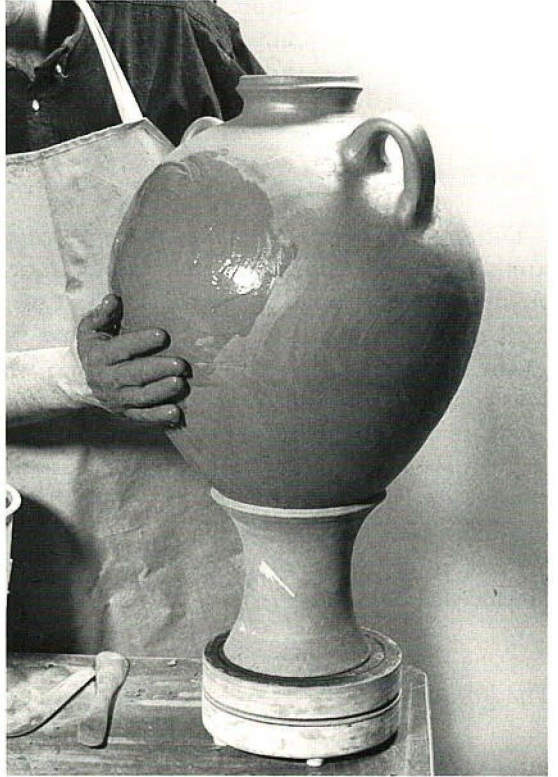
Fig. 16. Coating the vessel with a slip.
