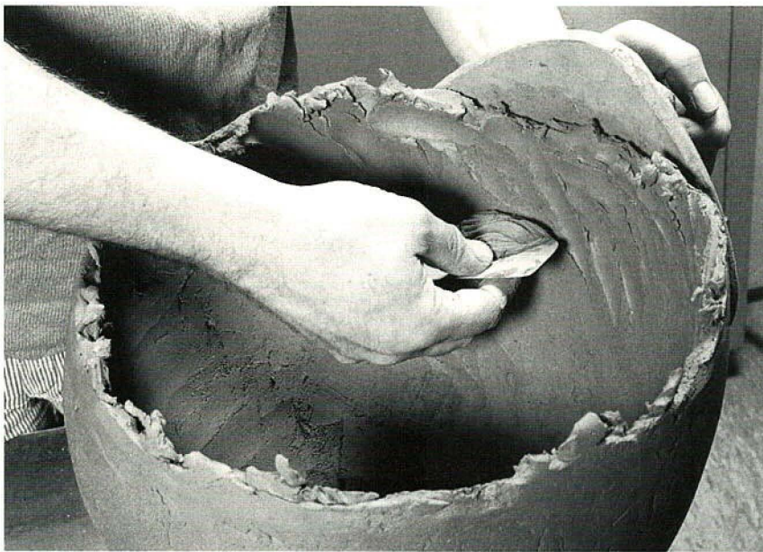
Fig. 11. Thinning the wall with a rib.
