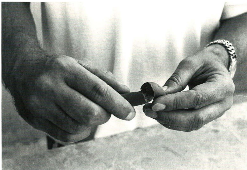
Fig. 3. Testing the cohesive strength by means of the potter's 'pigletstail' test'.
