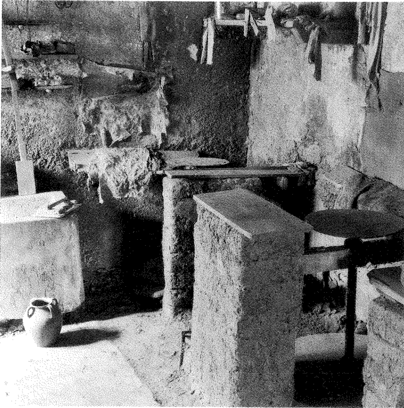
Fig. 4. Pabillonis, abandoned workshop, room 12: two of the three wheels and wetting tank.
